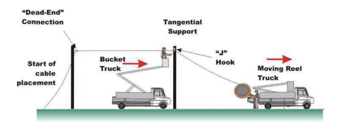
When using the moving reel method, operators must ensure that the aerial line truck or cable truck is about 10 to 15 metres ahead of the first pole position. This ensures that there is sufficient slack cable available for splicing and slack storage.
