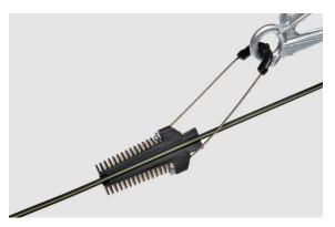
The formed wire dead-ends function by gripping the cable uniformly over the length of the support, typically two to four feet in length. For this reason they are often seen as the strongest solution for long spans. The alternative wedge clamp dead-end works by anchoring the cable between opposing wedge blocks, gripping a shorter distance of cable; perhaps only 15 to 30 cm. Wedge supports are perhaps better suited to scenarios where strain is less of an issue and spans and below 100 m.
