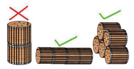
If storage place is limited and it becomes necessary to stack, then stack the completely wrapped on their flanges. Stacking is allowed only for the drums whose flange diameter is 125 cm or less. Do not store drums on flat flanges
