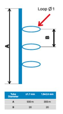
If the cable in the lower part directly enters into the connector panel, it should enter by three loops. The purpose of this is to compare the change in the lengths of cables given the change in temperatures. This is from the lower part of the panel.
