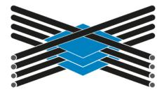
Prior to taking the cable from the figure 8, tilt it by 180°, with the aid of other persons, so that the beginning of the cable is facing upward. After pulling it through, **do not wind it back up onto the drum**, but place it back in a figure "8" for further laying.
