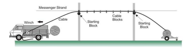
It is vital that the pulling winch is calibrated to stop the operation when the installation tension exceeds the maximum rated cable load (MRCL). If this type of winch isn't available, a dynamometer can be used to monitor installation tension. The dynamometer must be equipped with an audible alarm or visual display that allows the pulling operation to be stopped when the installation tension reaches the MRCL.
